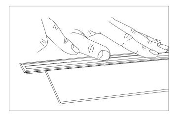
4. If you need to cut the tile...Measure where the cut needs to be and mark on backing paper.
