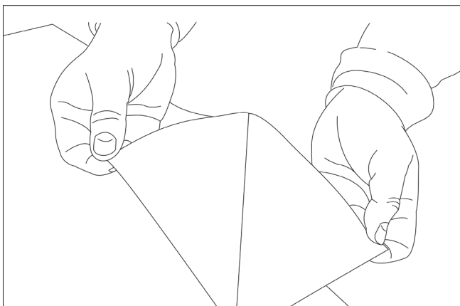
4. Peel back around 30cm of the backing paper and apply the sticky side to the top of the wall, allowing a little excess to overlap the ceiling
